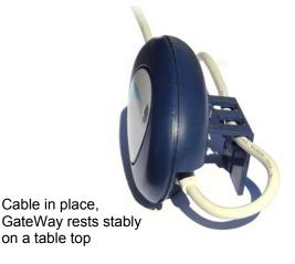
Once the cable is installed, the GateWay is ready to set-up and run your measurement network from your DataLink software. Please note that DataLink will not function without being connected to the GateWay.
